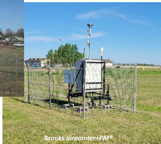
Figure 2. PAS Continuous Air Quality Monitoring Stations
