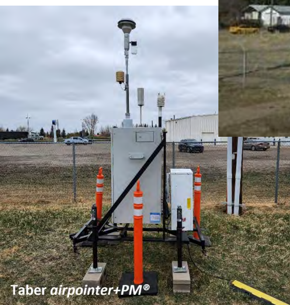
Figure 2. PAS Continuous Air Quality Monitoring Stations
